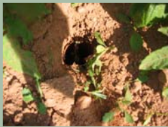
Fig. 1. Bulk density core sample
